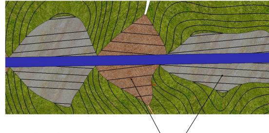
In a sloping road the lines on the cut/fill surface will always be at an angle to the edge of the road
